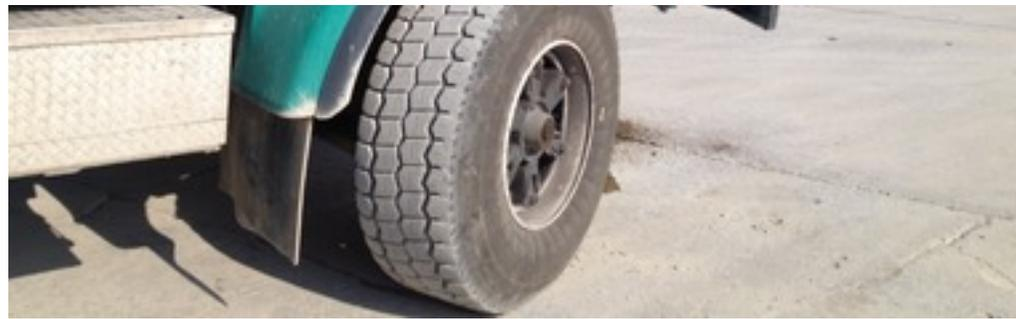
*The [GT876](#) is as tough as nails, which is good because Williamson County Ready Mix runs over nails, rebar and just about anything else you can find in a construction yard. Company officials say this GT Radial mixed service tire is one of the best for resisting cutting and tearing.*
