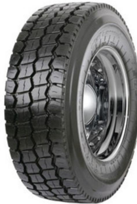
Designed for heavy front axles, the [GT876](#) is an all wheel position, wide base radial that provides exceptional service in on/off
